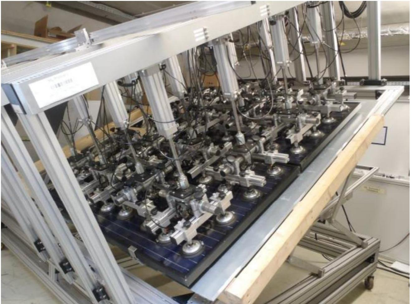
Fig. 2: system including PV-modules installed on test rig
